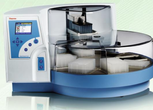
Figure 6. KingFisher<sup>™</sup> Flex for automated DNA extraction
