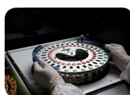
VIAL TRANSFER by mechanical tool from ALFRED 60 to HB&L
